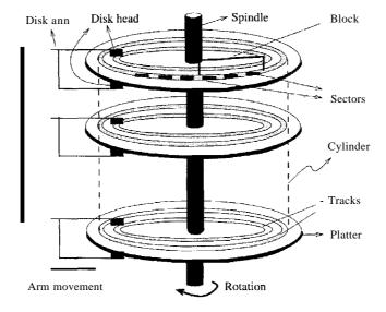
Figure 9.2 Structure of a Disk
