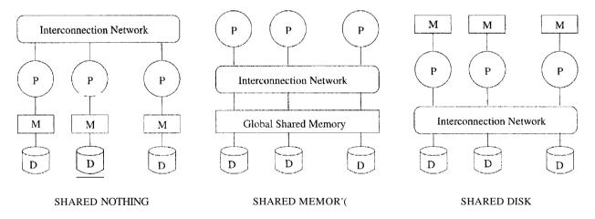
Figure 22.1 Physical Architectures for Parallel Da.tabase Systems
